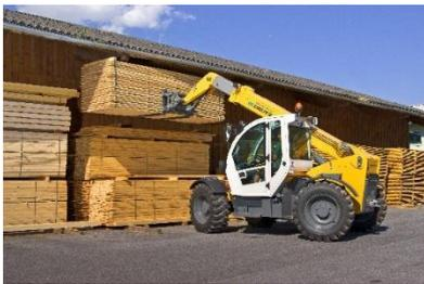
Caption: So as to provide a real-life illustration of how its e-drives perform in practice, DEUTZ has converted two telescopic handlers, one to a hybrid drive and the other to an all-electric drive.
