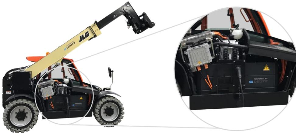
*Caption: The telescopic handler solution G5-18A, which was jointly developed by DEUTZ and JLG, uses a compact 360 volt drive system with two 40 kW electric motors – one for driving and one for the hydraulics in the telescopic arm.*
