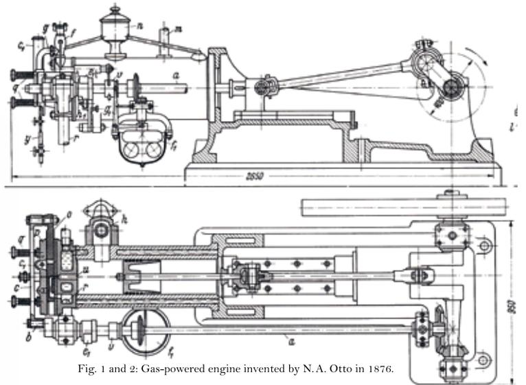
Fig. 1 and 2: Gas-powered engine invented by N.A. Otto in 1876.
