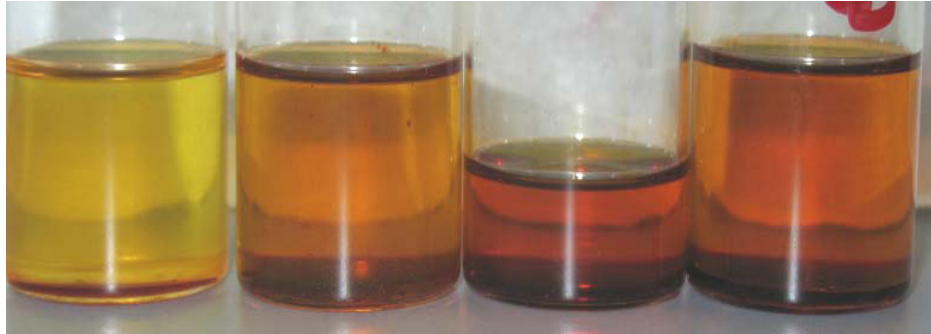
A 1 Change in pure biodiesel in storage at 50°C.
