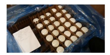
Freight Box: Double wall corrugated cardboard box Preservation: One VCI bag per box Parts stacked with cardboard layers and honeycomb cardboard.
