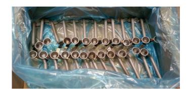
Freight Box: Double wall corrugated cardboard box Preservation: One VCI bag per box Parts per stacked with layers Up to 200 parts per box
