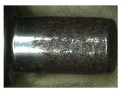
The surfaces have undergone significant attack and have a rough surface as though "eaten", usually irreparable
