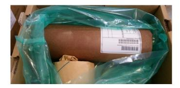
Rings rolled with VCI Paper, max. 100 parts per roll.
