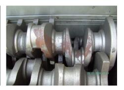
The surfaces are discoloured but not damaged. A cleaning or reworking is usually possible.
