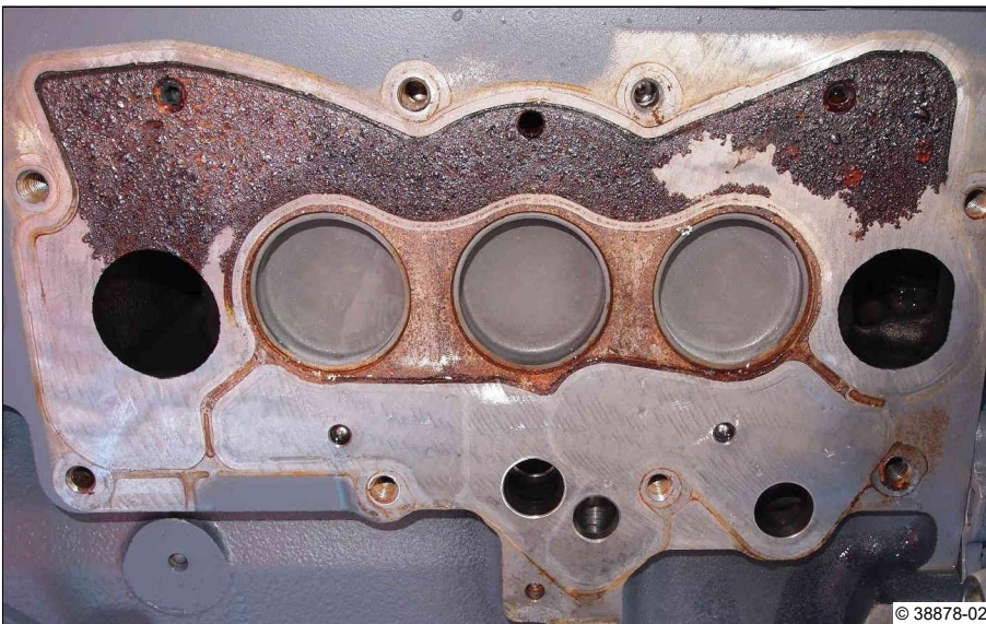
A7: Crankcase in the area of the lubricating oil cooler housing
