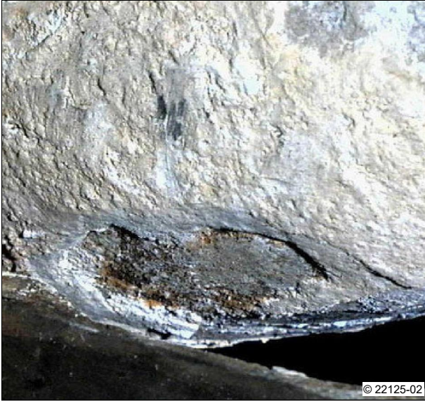
A13: Limescale deposits on a cylinder liner
