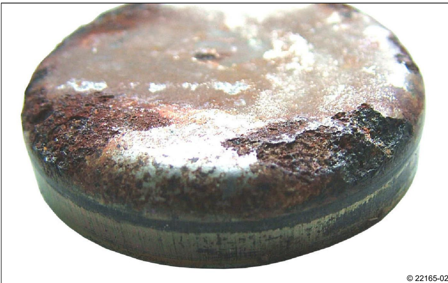
A11: Sealing cover, corroded
