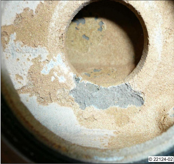
A12: Aluminium thermostat cover, corroded
